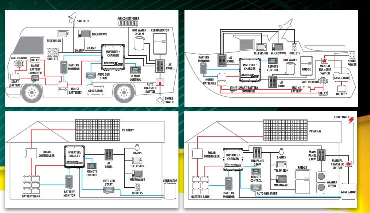
For reliable power, regardless of your application, the MagnaSine Inverter / Chargers, interconnecting system equipment and accessories are a solid base for back-up, or on-board power. Above are simple examples of how the MagnaSine system can fit into your application.
