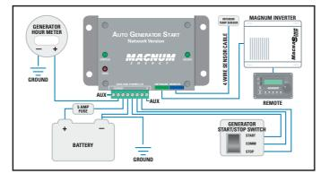
day, Battery state of charge, Battery voltage, High temperature or Inverter load amps. Also includes the ability to manually turn the generator on and off, generator exercise, warm-up and cool-down.
